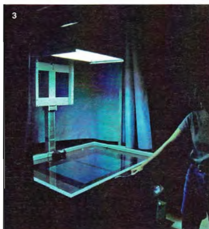
3 Expose the plate to light.
