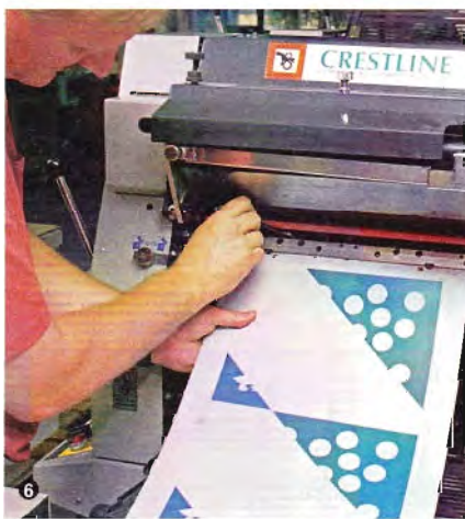
Mount the plate on the press.
