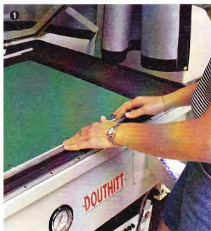
1 Insert the plate into the vacuum frame.
