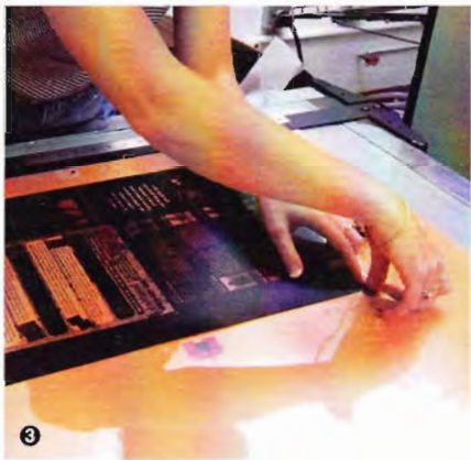
Tape the negative to the goldenrod paper.
