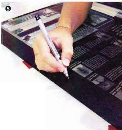
Cover any nonimage marks with opaque.
