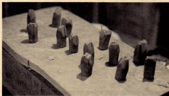
The Caslon punches for casting type, circa 1810, stored in the "Tomb" at the Stephenson & Blake foundry.
