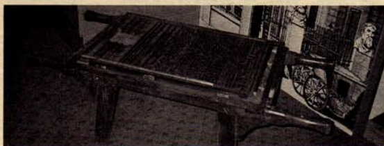
18th century "turtle" for moving composed forms to the press, formerly used at the Oxford University Press.
