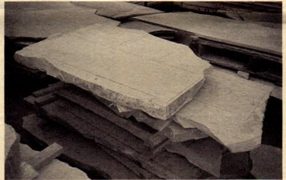
Stones quarried in Solnhofen ready to be chiseled to final size.
